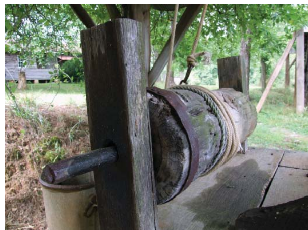
Figure 4. View of barrel component of well windlass.
