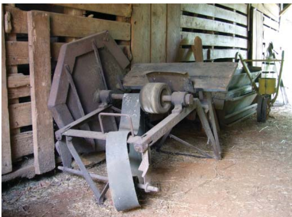
Figure 4. View of Hydes' portable circular saw, which was apparently used to saw much of the lumber for their buildings.
