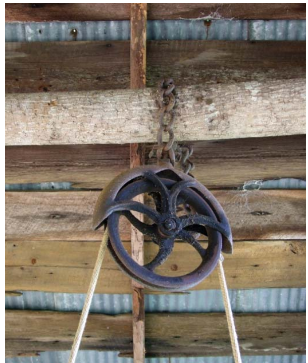
Figure 8. View of pulley component of well windlass.
